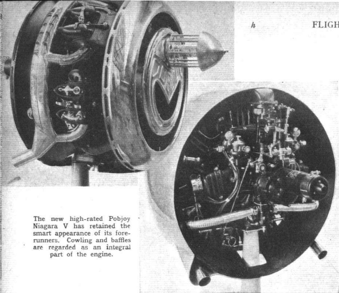
The new high-rated Pobjoy Niagara V has retained the smart appearance of its fore-runners. Cowling and baffles are regarded as an integral part of the engine.
